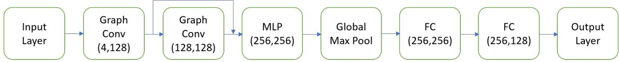
Figure 3: The architecture of our neural network: each vertex initially has four node attributes, namely the center coordinates and the radius of the corresponding ball; the two graph CNN layers extract features directly from the input layer of graph data and have 128 channels on their output; the multilayer perceptron layer concatenates and merges the node attributes from the graph CNNs; a global maximum pooling finds the largest value in each channel over all the nodes of the graph resulting in a shape feature vector with 256 elements; finally two fully-connected layers reduce the dimension of the feature vector and this dimension captures the number of classes.
