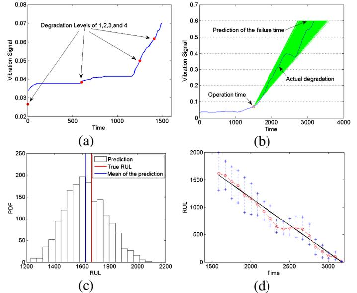
Figure 7: RUL prediction of the test unit #1
