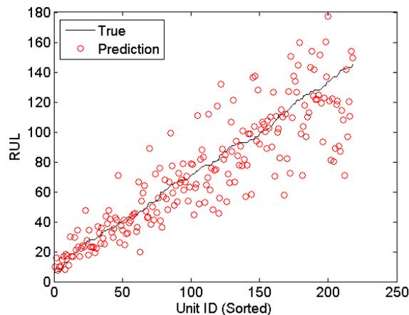
Figure 13: RUL comparison for 218 test units
