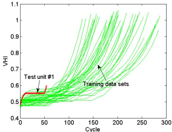
Figure 12: Training data sets for the test unit #1
