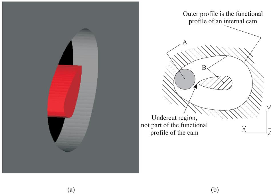
**Fig. 10** The loads applied on  $A$  are so that the outer profile of the cam is the one that is functional, although undercutting of  $A$  does occur for the inner profile.
