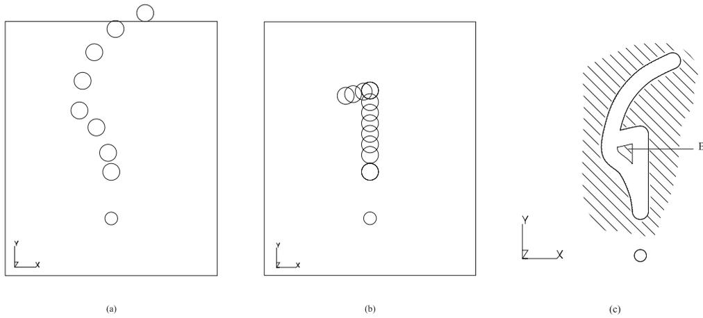
**Fig. 8** The discrete relative configurations of the striker  $A$  relative to the latch to be designed: the motion of the striker was separated into its “downward” motion (a) and its “upward” motion (b) because they correspond to different functions of the latch. Figure (c) shows the top view of the  $B_{max}^A$  forming the maximal triplet  $\langle A, B_{max}^A, M \rangle$ .
