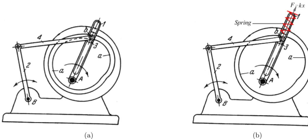
**Fig. 1** A link-gear fixed-slot cam mechanism from [2]. The slider 3, moving along the slot of link 1, has roller  $b$  fixed which slides and rolls along fixed slot  $a - a$  of special profile. The intermediate link 4 transmits oscillating motion to link 2 about fixed axis  $B$ .
