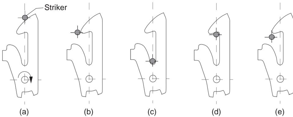
**Fig. 7** A secondary hood latch must engage and retain a vertically moving striker.
