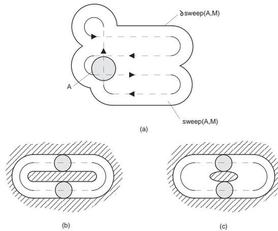
**Fig. 2** A conjugate triplet might not exist for given object and motion and this is illustrated in (a). If one conjugate triplet exists (b), there is an infinite number of conjugate triplets: (c) shows one more possible conjugate triplet for the case illustrated in (b).
