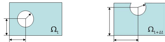
(a) A simple shape is parameterized by three dimensions that procedurally define the shape's boundary.
