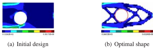
Figure 12. Strain energy distribution of the initial and optimal free-form shape with a circular hole as a moving obstacle. Grid size = 50 \times 25 .
