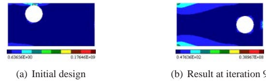
Figure 8. Strain energy distribution of the initial and optimal shapes of a rectangle with a circular hole. The design variables are the position of the hole. Grid size = 50 \times 25 .
