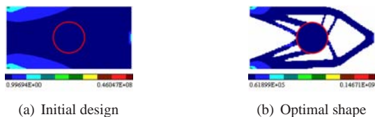
Figure 13. Strain energy distribution of the initial and optimal free-form shape with a disk as an attachment. Grid size = 100 \times 50 .
